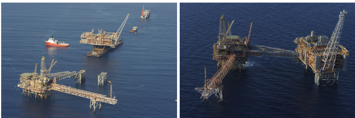
The North Rankin B topsides on Heerema's H851 barge are carried and set-down into position.
