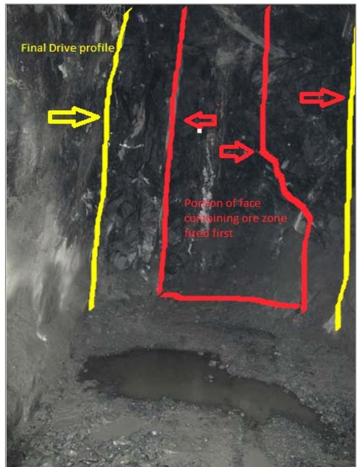
Figure 4: Resue' Cut showing original face and ore only portion of face fired and bogged
