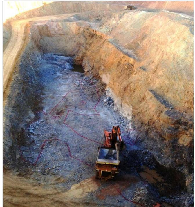
*Figure 2: Empress pit showing final floor in far wall under ramp. Ore zones in red paint. Pit has a further 12 metres vertically of ore to be mined from the point shown in the figure.*
