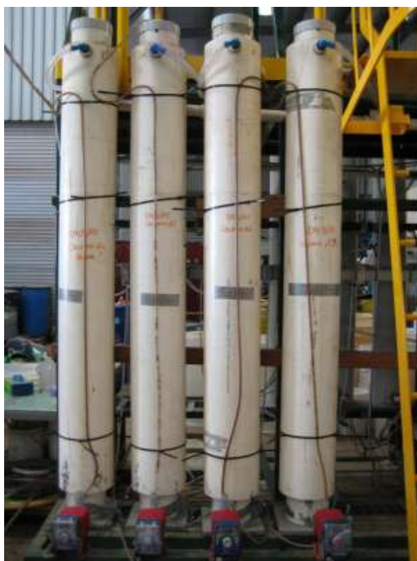
Häggån bacterial heap and tank leach testing at SGS Lakefield Orestest, Perth
