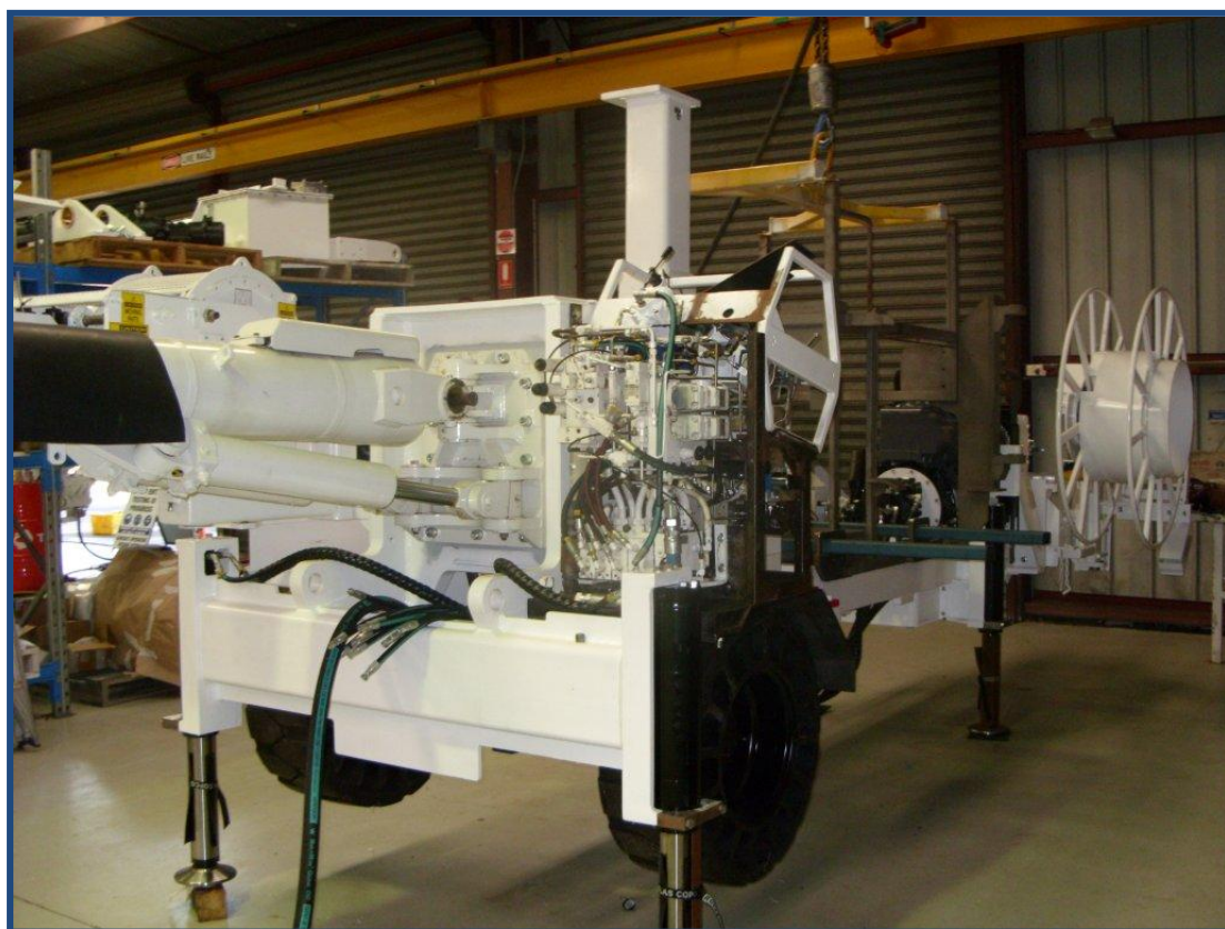
Fig 1. New, in-house Swick Mobile Underground Diamond Drill Rig taking shape
