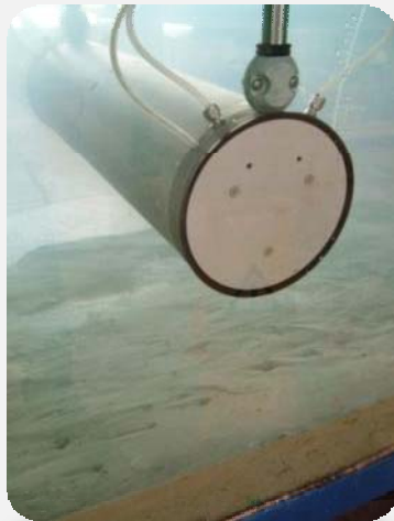
O-Tube Test Facility Pipe Stabilisation
