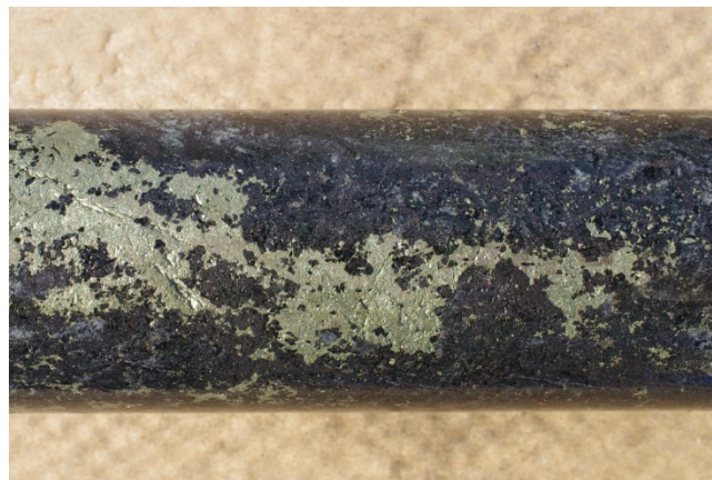
Figure 2: Close-up of coarse chalcopyrite magnetite mineralisation in diamond drill hole EHRC404 diamond tail.
