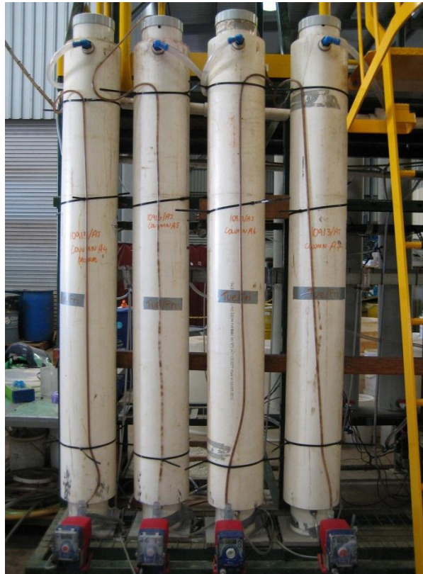
Häggån bacterial heap and tank leach testing at SGS Lakefield Oretest, Perth
