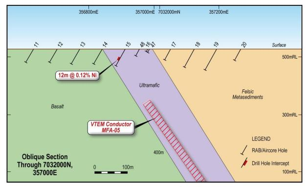
Figure 2: RAB/Aircore Drill Section, Fisher East, looking NW
