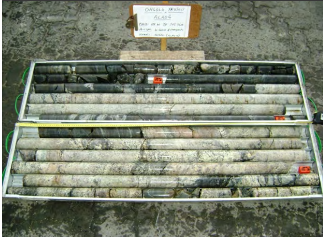
Figure 10 MS7 Mineralisation in drillhole ALAD6 – Alaskite in contact with biotite-gneiss with minor skarn development.
