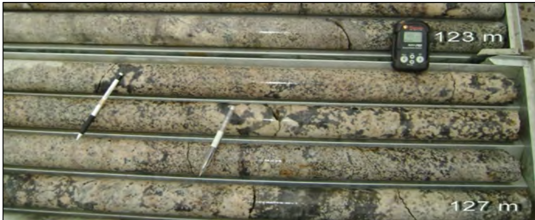
Figure 7 High grade alaskite mineralisation with smoky quartz in diamond drillhole ALAD001
