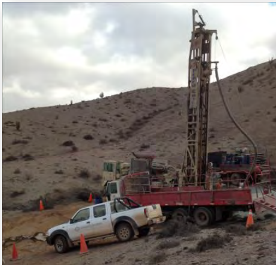
RC drill rig at Simpson (August 2012)
