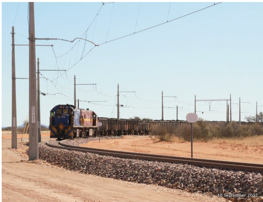
Tshipi Borwa rail siding trial with 208 wagon train
