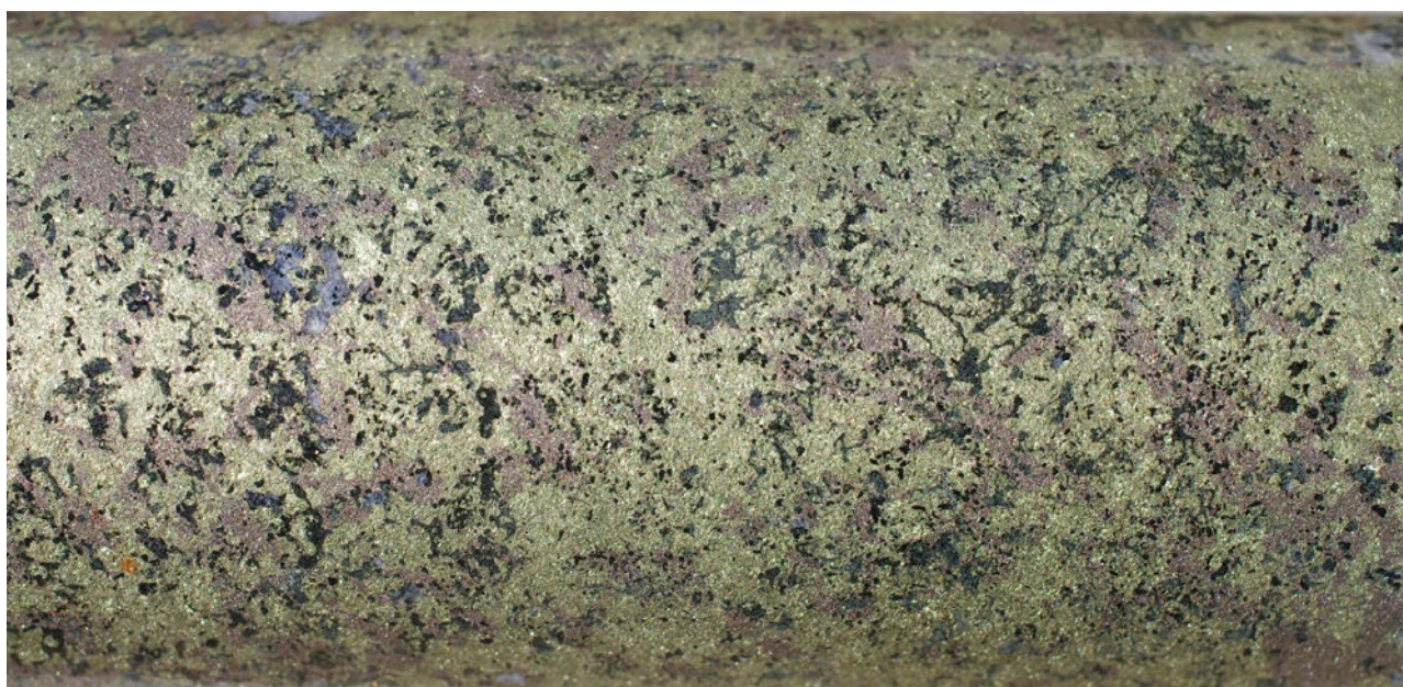
Close-up of massive sulphides intersected in diamond drill hole EMCDD056.
