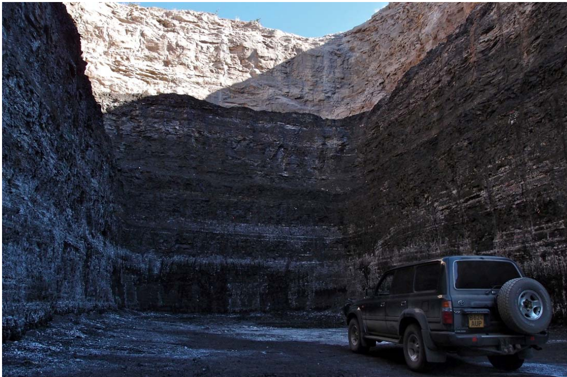
Sese coal seam (18m thick) with 15m barren cover exposed at the Sese Bulk Sample Pit in PL96/2005
