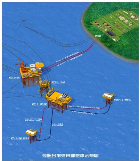
Schematic of Block 22/12 development project and CNOOC processing and export system
