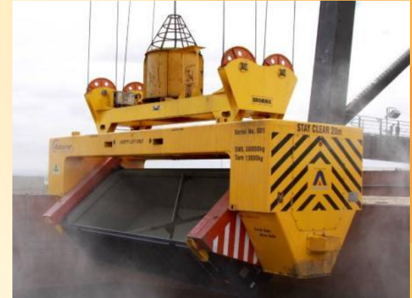
Port Adelaide – custom ship loader
