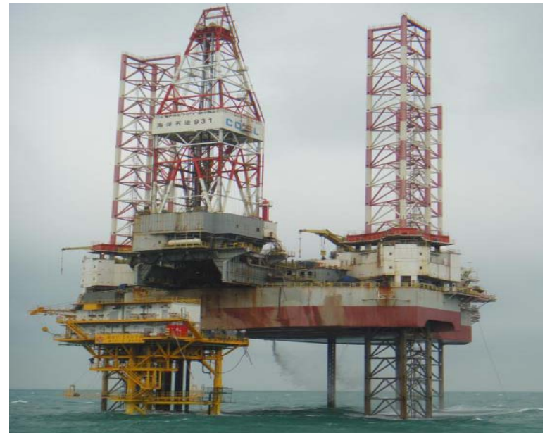
COSL HYSY 931 jack-up rig drilling over WZ 6-12 platform
