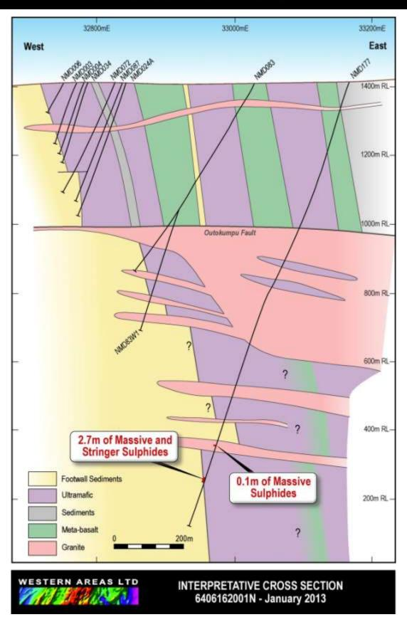
Figure 3: Interpreted cross section (25,355N) at New Morning showing approximate location of NMD 177
