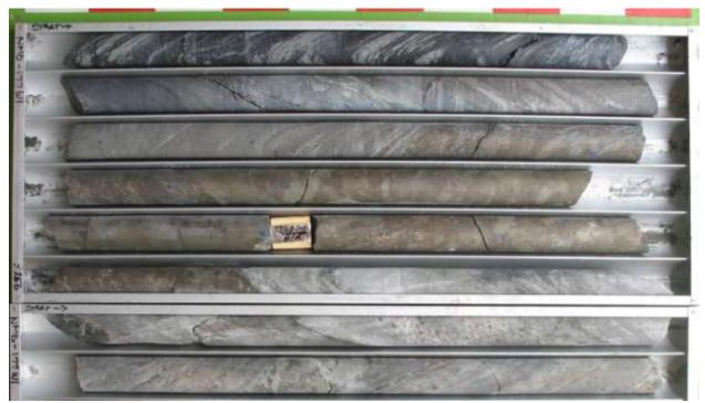
Figure 1: Mineralised drill core from NMD 177 showing massive nickel sulphides
