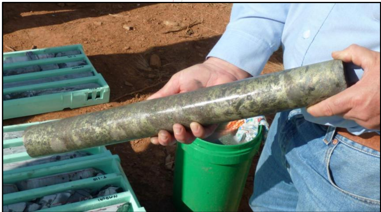
Massive sulphide mineralisation - Nymagee Copper Deposit
