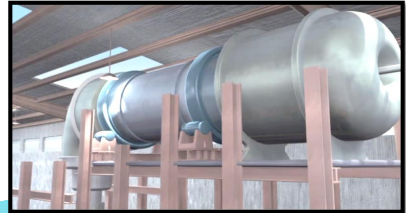
Central Processing Plant: Yellowcake Drying and Packaging Unit
