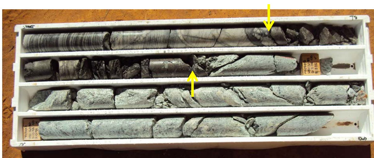
Figure 5: MFED013 Core Tray showing 0.7m massive sulphide intersection (between yellow arrows)
