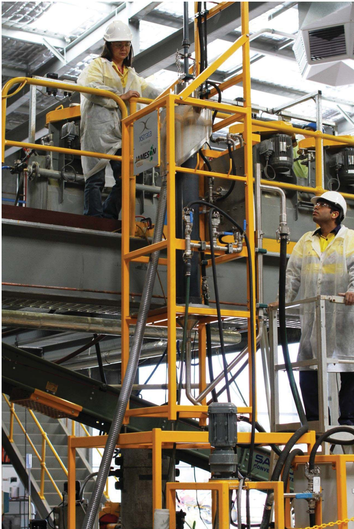
The pilot plant scale Jameson Cell, ready for action.
