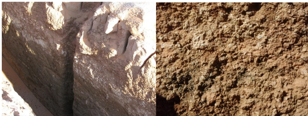
Trench through Reguibat calcrete uranium deposit showing the granite pebbles that are discarded in the screening tests
