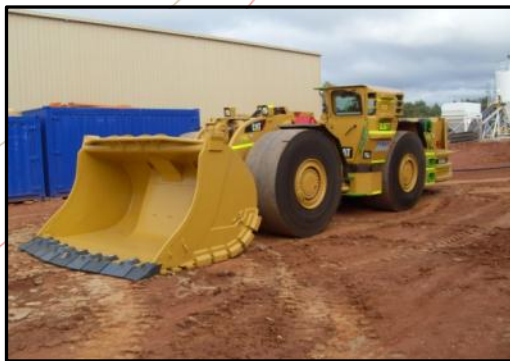
Delivery of new Elphinstone R2900 Loader
