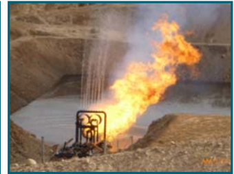
Open hole test of lower zone of Taza 1 well, Kurdistan
