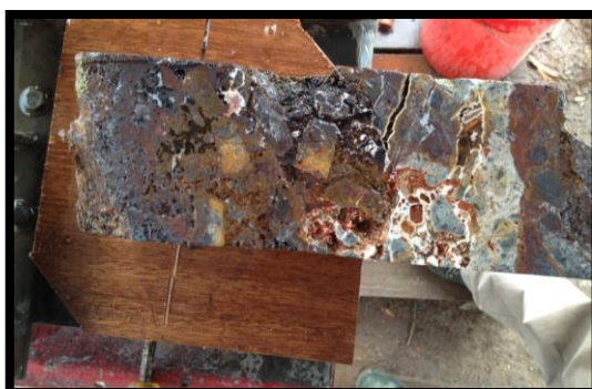
Photo 4. Gossanous (after sulphide), quartz-flooded breccia: Advene (Josephine Moulder) lode
