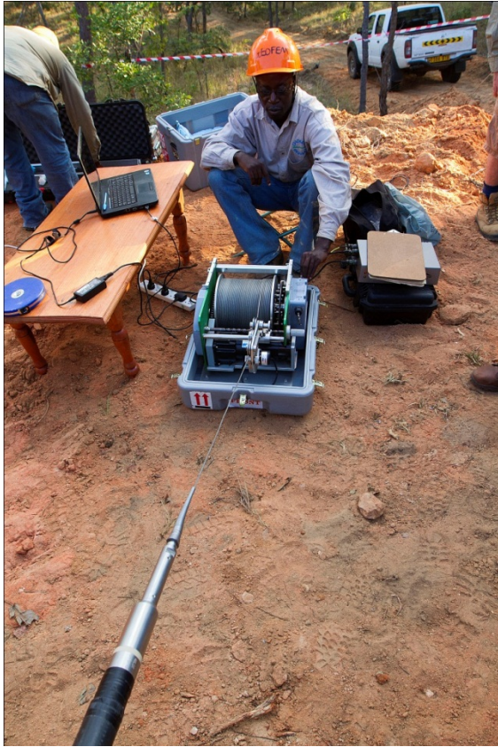
Figure 3: EAF Geologist operating down hole logging equipment
