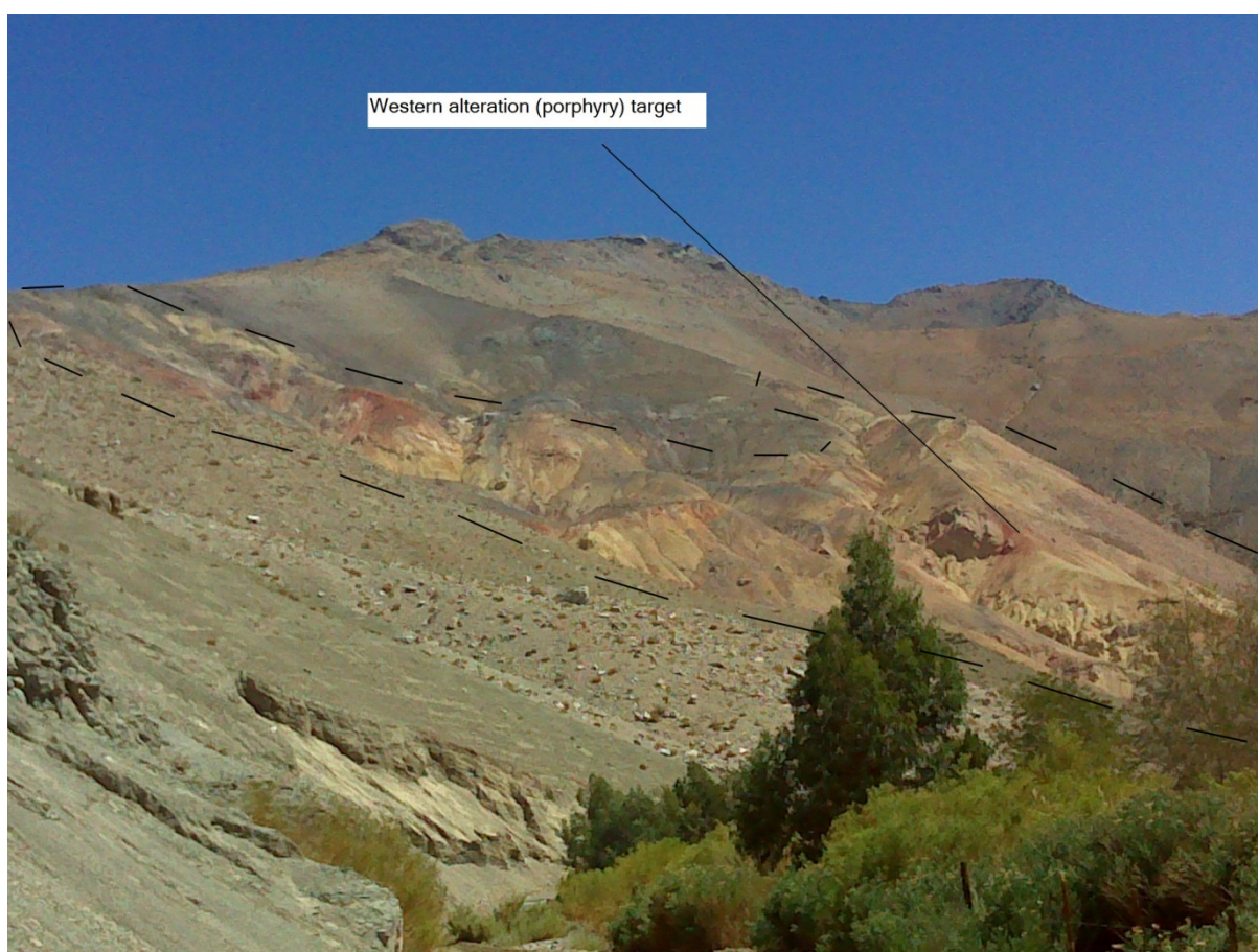
Figure 5. Timon Project, southeast in the valley of the Rio Jorquera looking north, secondary exploration target prominent alteration (argillic with iron oxides) in Triassic volcanics representing a buried intrusive porphyry.
