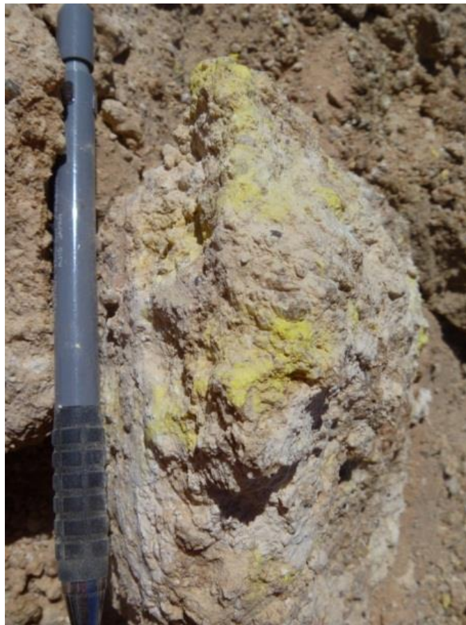
Trench through Reguibat calcrete uranium deposit showing the patches of yellow uranium mineralisation
