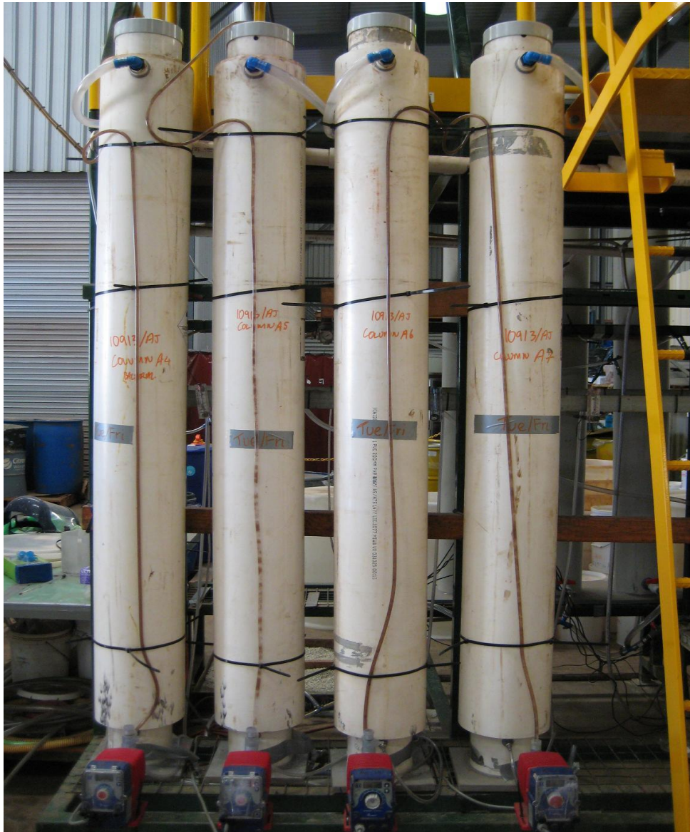
Two metre bioleaching testwork columns at the SGS Laboratory in Perth, Australia
