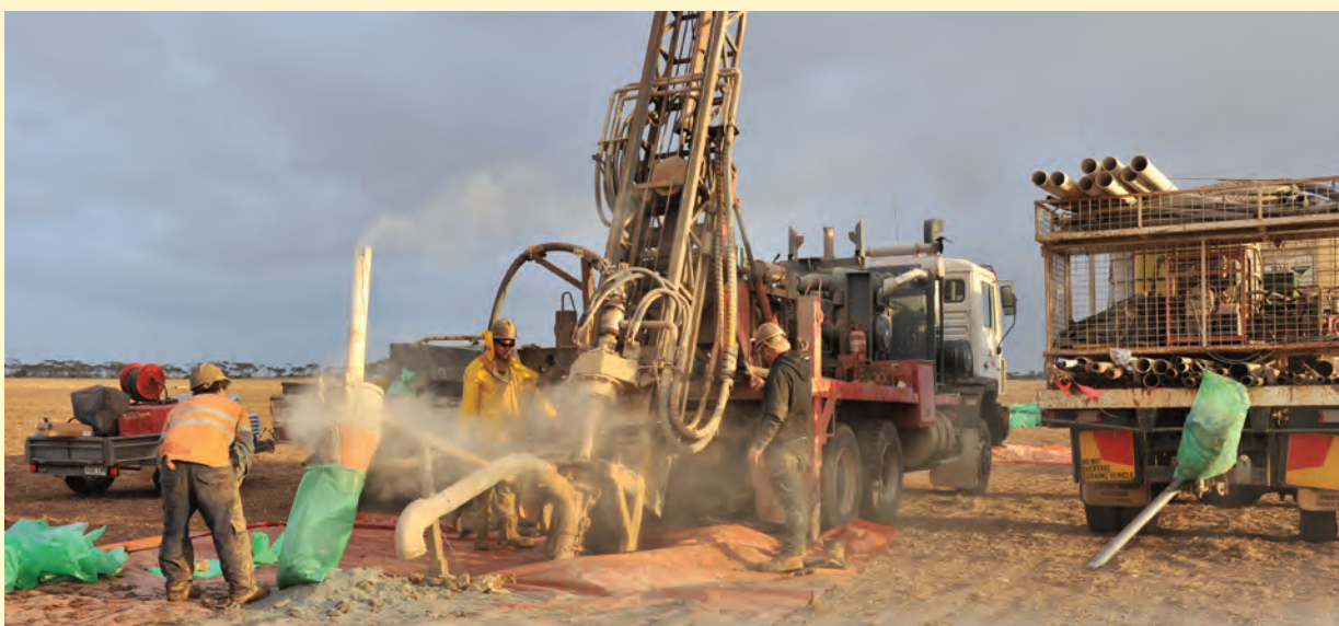
2013 aircore drilling on the Alford West prospect, Moonta Copper Gold Project.
