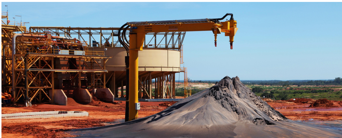
Initial HMC stockpile following commissioning of the mining unit and wet concentrator plant
