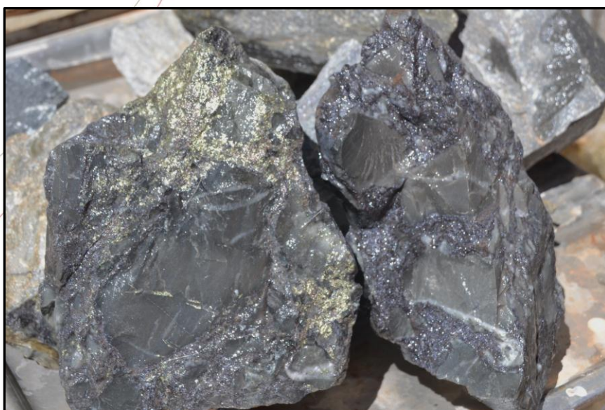
Samples of strong zinc-lead and copper sulphide mineralisation from the first cross cut into the Hera ore body
