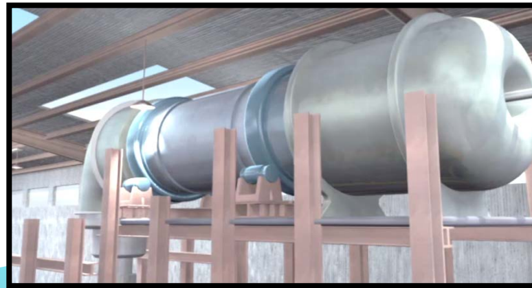
Central Processing Plant: Yellowcake Drying and Packaging Unit
