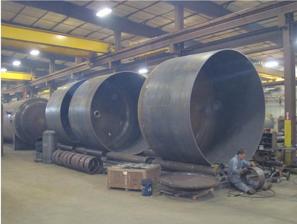
Figure 2: Ion Exchange Columns for Peninsula's Ross CPP, Wyoming USA
