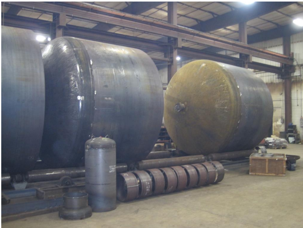
Figure 3: Ion Exchange Columns for Peninsula's Ross CPP, Wyoming USA
