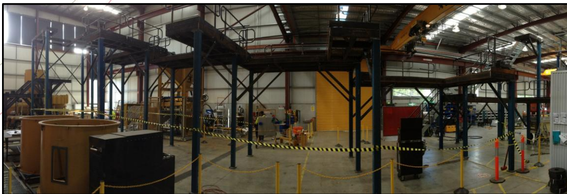
Rougher float frame assembly nearing completion. at Gekko Systems factory in Ballarat
