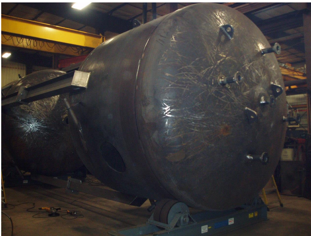
Figure 5: Ion Exchange Columns for Peninsula's Ross CPP, Wyoming USA
