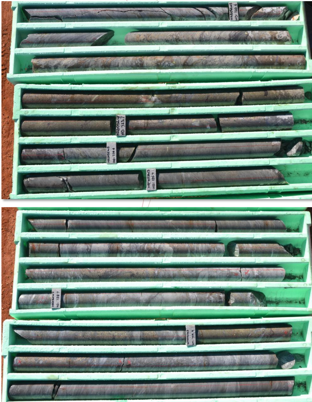
Core photos of strongly mineralised interval in hole HRD052W3
