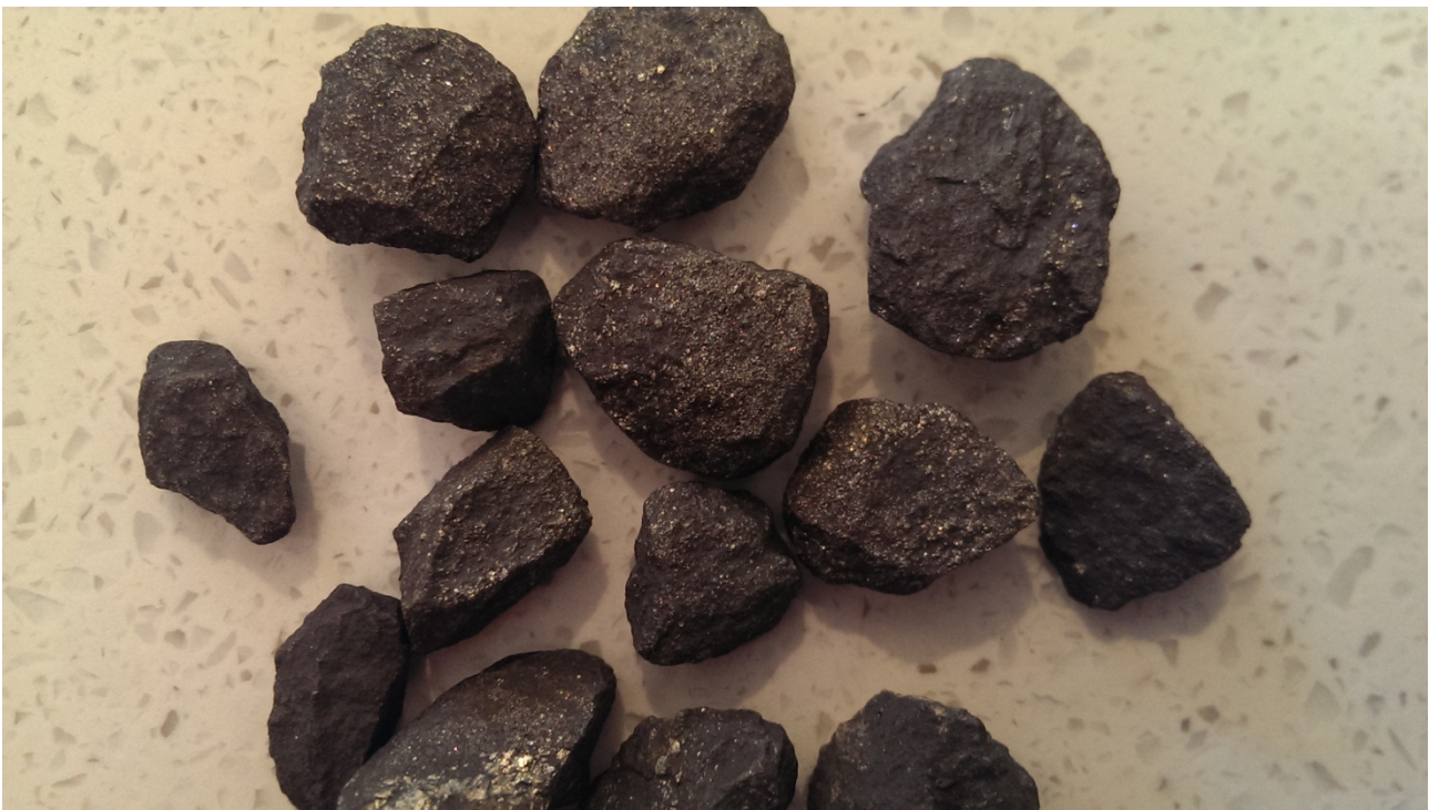
Figure 2: Close up of drill chips from RC hole MFEC065 (2m @ 8.1% Ni) at Musket. Pentlandite, a primary nickel sulphide mineral (\text{Ni,Fe})_9\text{S}_8 , is prevalent.
