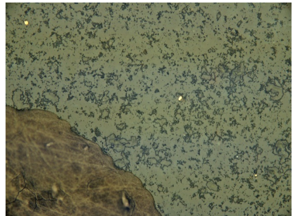
Plate 4: This view from a quartz-sericite-gold band captures three tiny grains of gold (top left, centre, bottom right) that are between 5 and 10 microns in size. ( SW Limey Dam Prospect 5177005mE, 7731200mN Photo approx. 1mm wide ).
