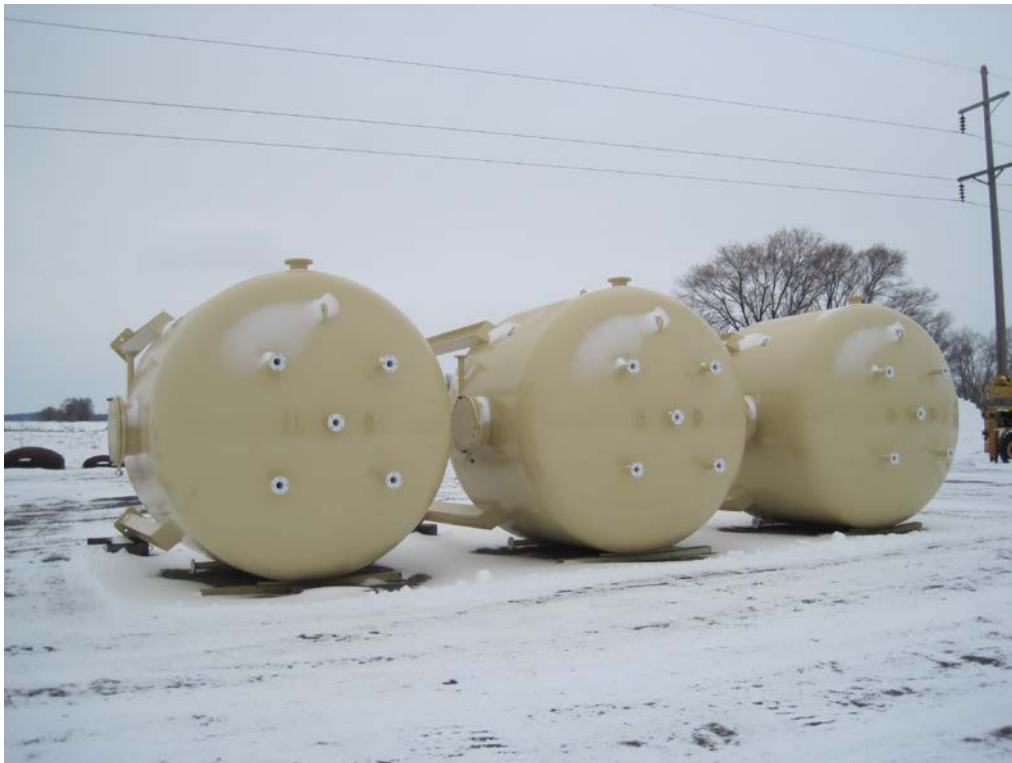
Figure 2: Completed Ion-Exchange Columns for RPA
