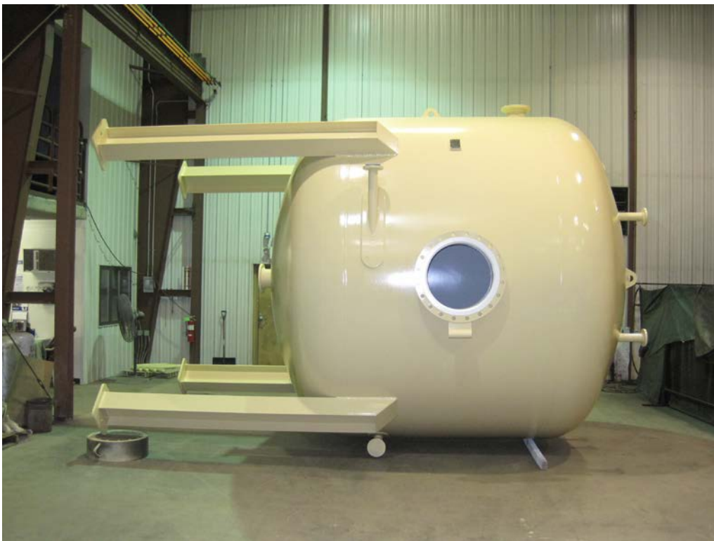
Figure 3: Completed Ion-Exchange Column for RPA
