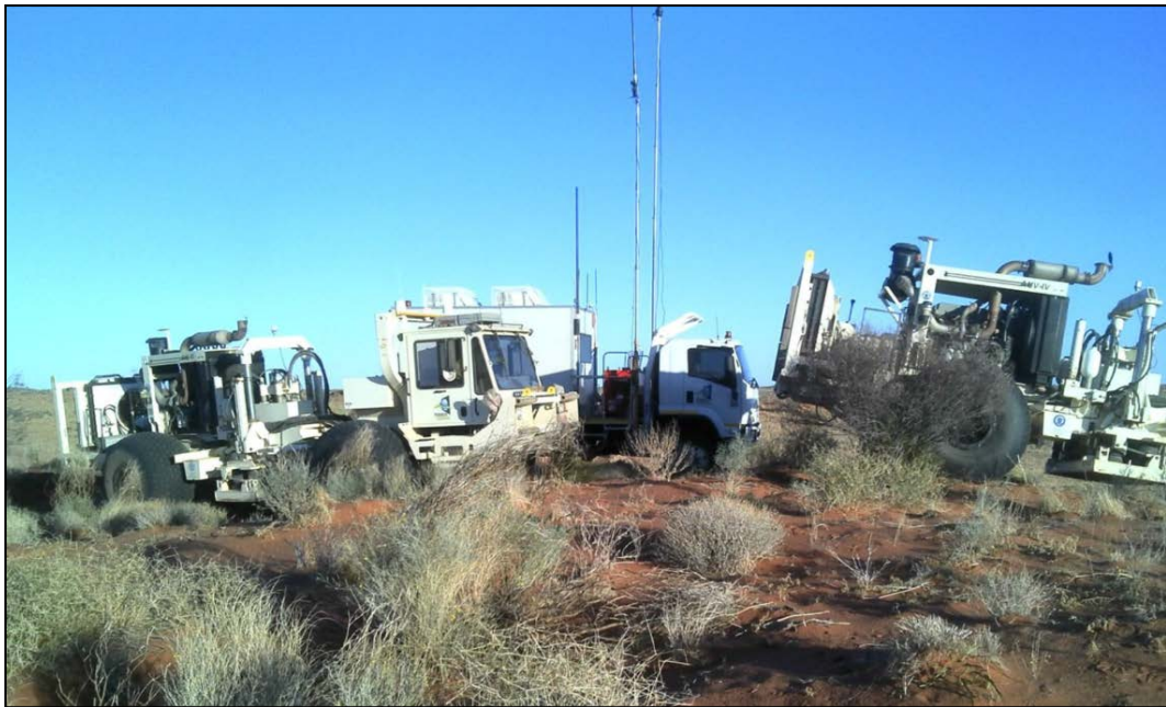
Vibroseis trucks providing sound wave source as it passes the recording truck.- Dundinna 3D Survey
