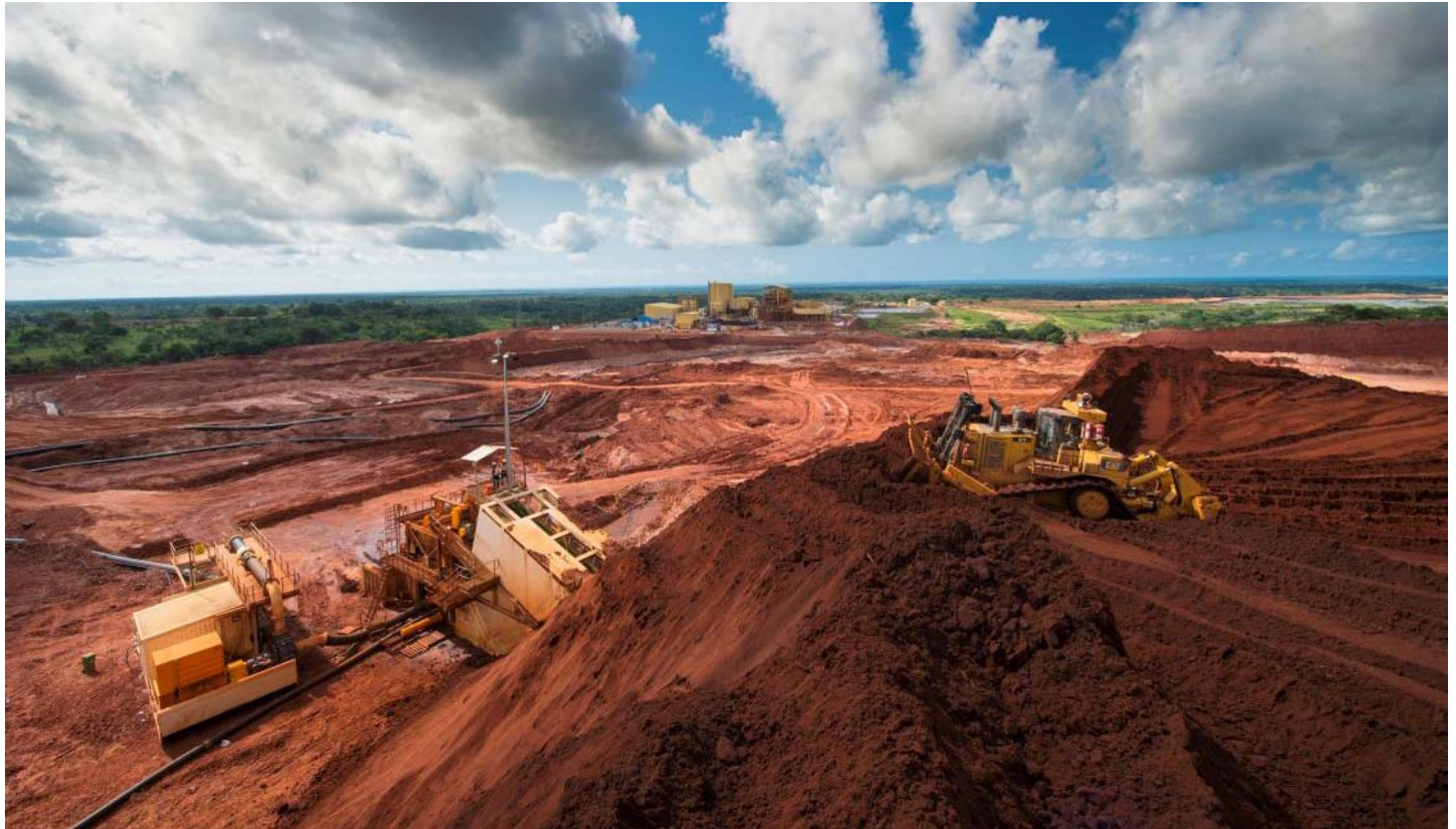
Kwale mining operations and dozer trap mining unit
