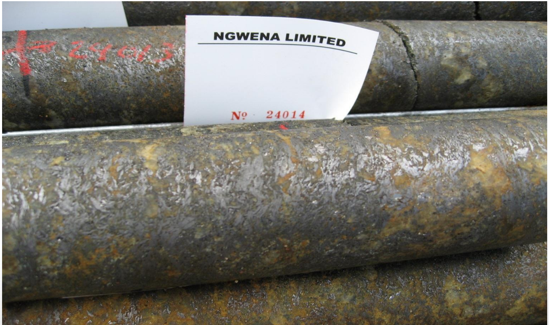
Drill core from Ntaka Hill (20km SW of Chilalo) showing coarse flake graphite
