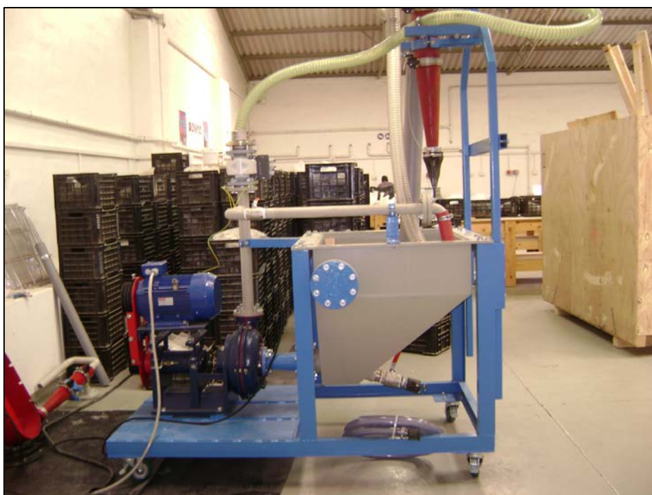
Figure 4: Schauenburg Pilot Plant in RUN's Laboratory
