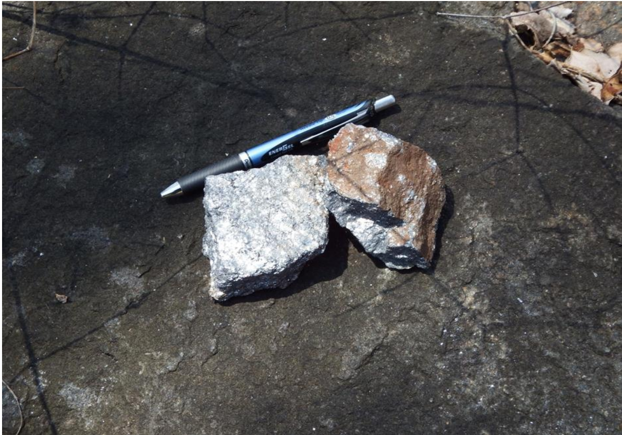
Figure 4: Coarse flake graphite in Chilalo rock chip
