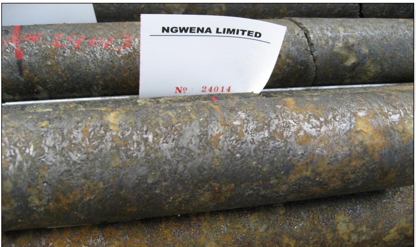
Figure 3: Graphite in diamond drill core from Ntaka Hill (NRD09-016, 188m)
