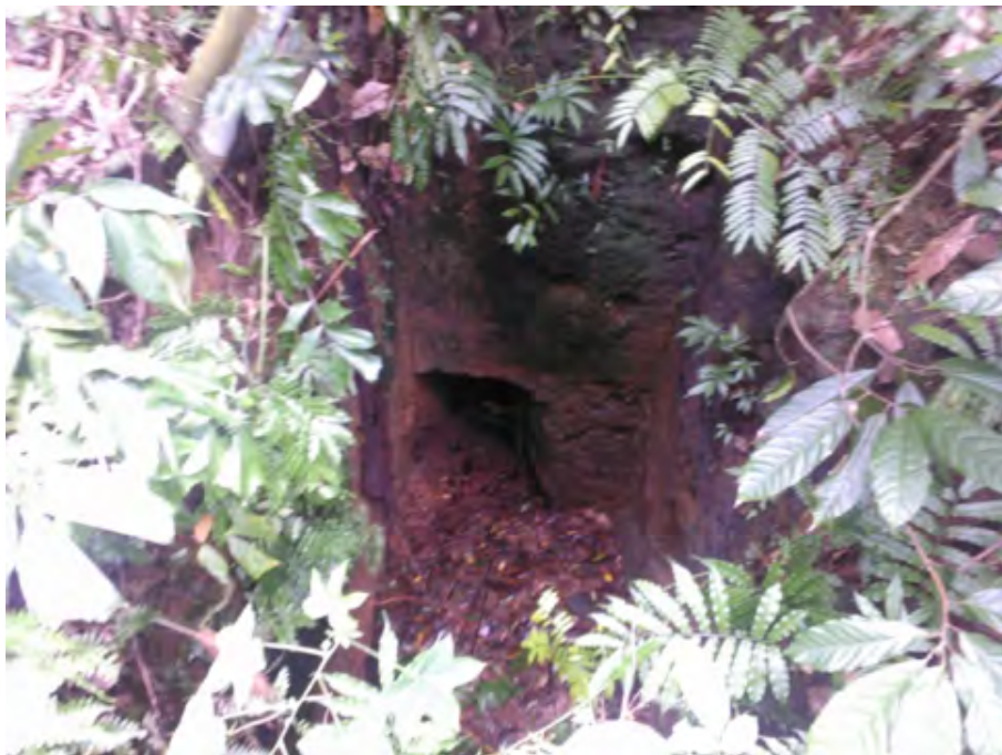
Figure 17: Vertical Shallow Shaft in EL237 with Horizontal Excavation possibly to follow a Vein
