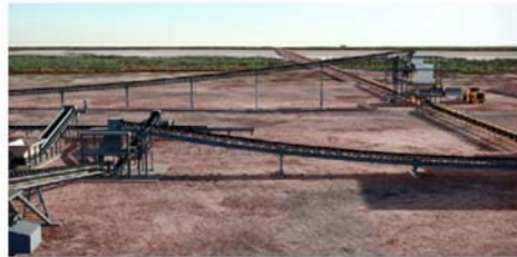
The highly automated stockyard, with a stacker and reclaimer, will load the TSV via the conveyor
