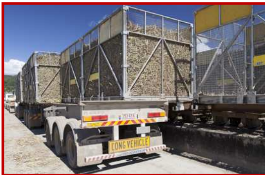
Sugar Cane Transfer Units (53 units sold to QUBE) Showing side shifting of cane bins onto rail cars
