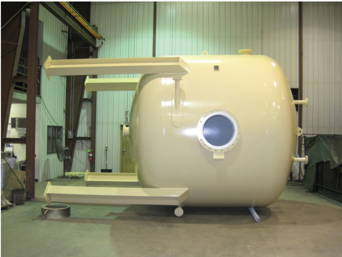
Figure 3: Completed Ion Exchange Column for the CPP
