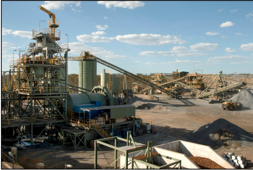
Lake Johnston Operation showing the milling circuit in the foreground and the crushing circuit in the background
