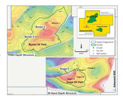
Interpretation of the 257 km, 2D seismic survey acquired in the Sumbagsel PSC (Cooper Energy 100%) is complete. The survey delineated a number of leads and identified some new targets for future evaluation.
